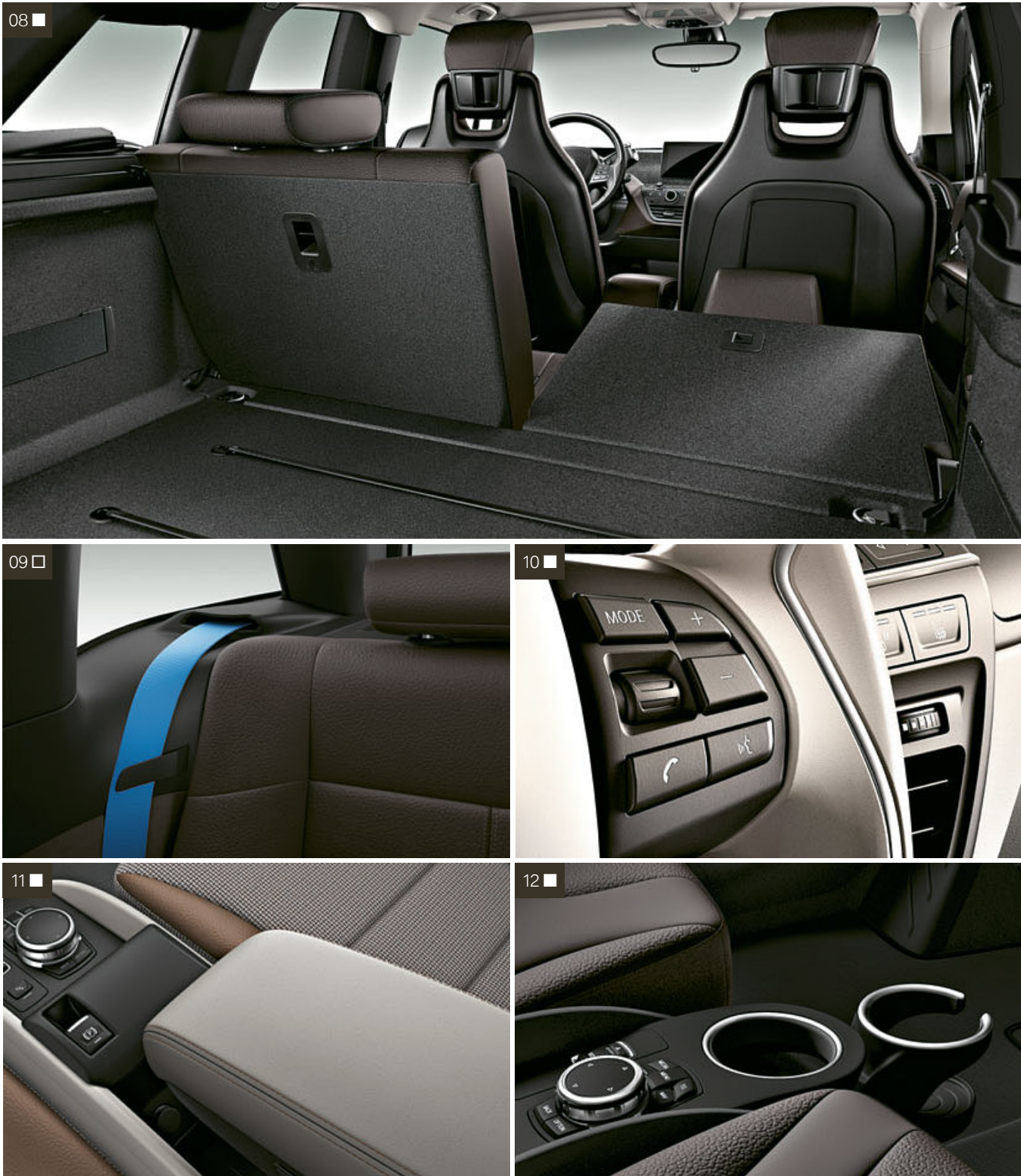
[08] The backrests can be folded down in a 50:50 ratio and each side can be set to one of three positions, as required. [09] The seat belts for all four seats appear in BMW i Blue. They provide the same functionality as the standard three-point seat belts. [10] The multi-function buttons for the steering wheel can be used to operate the telephone settings, audio and
